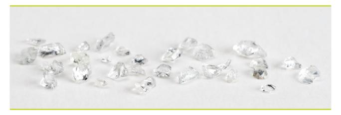
GLASS GRIT ST is a fine blasting abrasive in accordance with DIN 8201, based on broken sodium glass. The product meets the work protection requirements in accordance with DGUV rule 100-500, part 2, chapter 2.24, "Working with blasting equipment (blasting work)".
